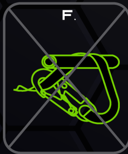
To any object which is shaped or dimensioned such that the snap hook or karabiner will not close and lock, or that roll-out could occur.
