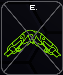
Directly to webbing or rope lanyard or tie-back (unless the manufacturer's instructions for both the lanyard and connector specifically allow such a connection)
