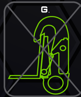
Do not use connector on an anchorage object in the manner depicted in picture-G
