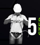
Connect chest strap and position in mid chest area 6" (152mm) to 8" (203mm) below the trachea but not below the sternum. Tighten to keep shoulder straps taut.
