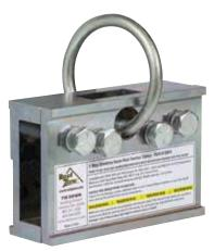
Zinc-Plated Steel Anchorage Device Galvanized O-Ring: 3.75" Round Galvanized O-Ring Thickness: 0.4" Anchor Size: 2" x 4" x 6" Base Thickness: 3/8" Bolts: 1/2"-13, 2-1/2" Grade 5 with 1/2" Lock Washers
